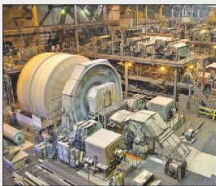
Above left, a grinding mill at the Tilden Mine is shown. There are a dozen mills at the mine, each drawing roughly 5,700 horsepower, electrically operated. The mills are part of the huge draw of electrical power needed to process raw ore into iron ore pellets. Similar mills are also used at the Empire Mine. (Photo courtesy of Cliffs Natural Resources) Above right, staff is shown performing open heart surgery at Marquette General Hospital. Hospital officials said funding for staff and development at the hospital could be negatively affected in light of potential electricity cost increases. (Photo courtesy of Marquette General Hospital)
